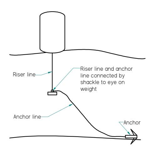
Attach the Riser Line to the Weight via the shackle through the eye in the Weight. At the same time attach the Anchor Line to the same shackle and ensure that the Anchor is securely attached to the other end of the Anchor Line – see drawing.
